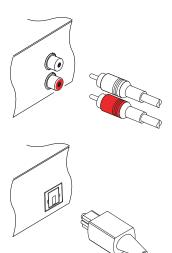
You will need to obtain an audio cable (RCA cable) to connect the audio connectors. Plug one ends of the cable into the AUDIO L (white) and AUDIO R (red) sockets on the digital receiver, and the other ends into the matching sockets on your television or audio system.
